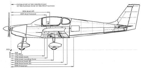
The method of calculation of the aircraft empty mass, total aircraft moment, centre of gravity and percentage mean aerodynamic chord appear from formulae set out in the table and the formulae below.
